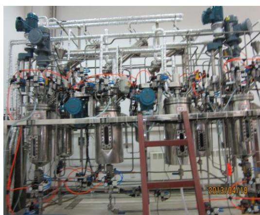
Fig.8 An experimental equipment for tar separation
