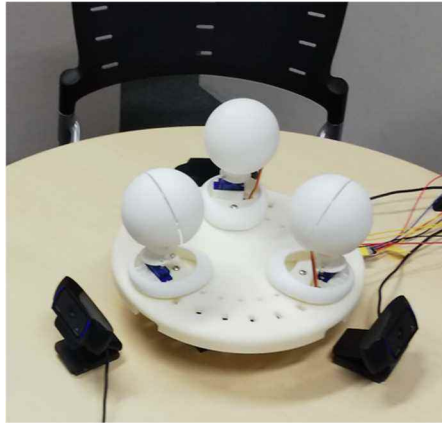
Figure 1. Table-top robot system prototype using specialized face-tracker software to ‘mimic’ users’ non-verbal behaviors.
