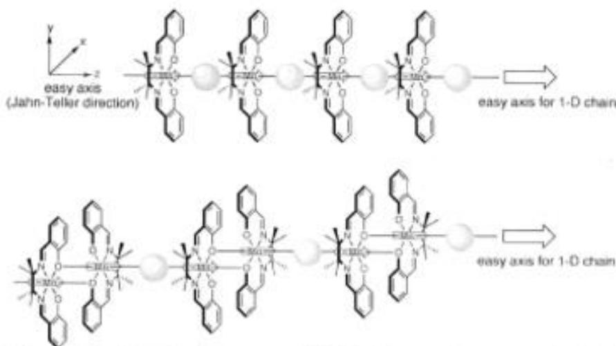
Figure 1. Schemes of one-dimensional arrangements of MnIII saltmen units (monomer and out-of-dimer forms) with linkers (green ball; organic linkers or coordination-donor metal complexes). The Jahn-Teller axis of MnIII ion is directed along the chain direction, producing an easy-axis for 1-D chain (Ising-type axis).
